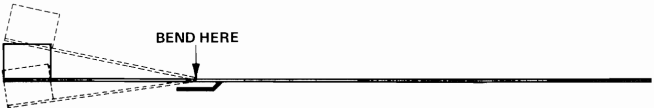
Figure 4-6. RHODES Damper Arm — Alignment Adjustment
